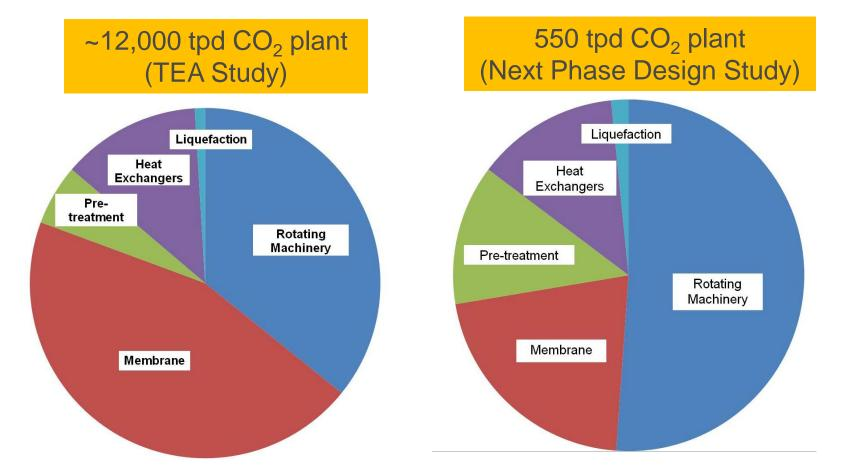
Further membrane bundle cost reduction is essential for larger systems by manufacturing process optimization
